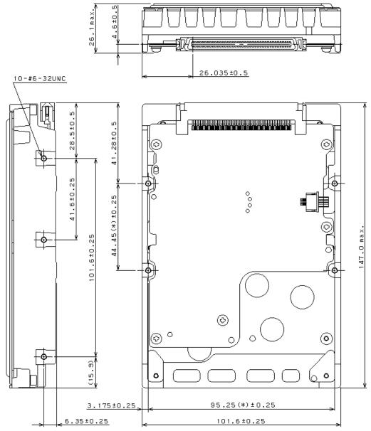
The value marked with (\*) indicates the dimension between mounting holes on the bottom face.
